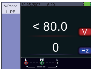
Standby Screen for the Voltage and Frequency
