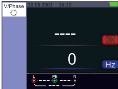
Initial Screen of the Phase Sequence Measurement
