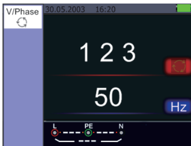
Phase Sequence Screen When connected in clockwise direction
