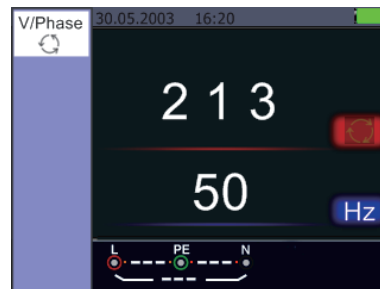
Phase Sequence Screen When connected in counter-clockwise manner
