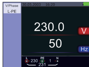
Screen While Measuring Voltage and Frequency
