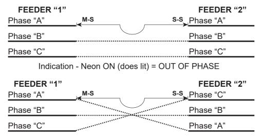
Note that the links must be arranged so that the phases are Connected in Phase, as indicated by the dotted lines. Do Not Use Phasing Sticks unless you have been fully trained In High Voltage work and understand the system fully.
